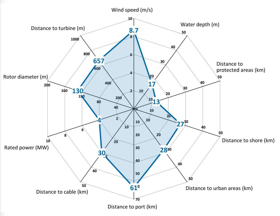
Properties of the current global offshore wind turbine fleet.
