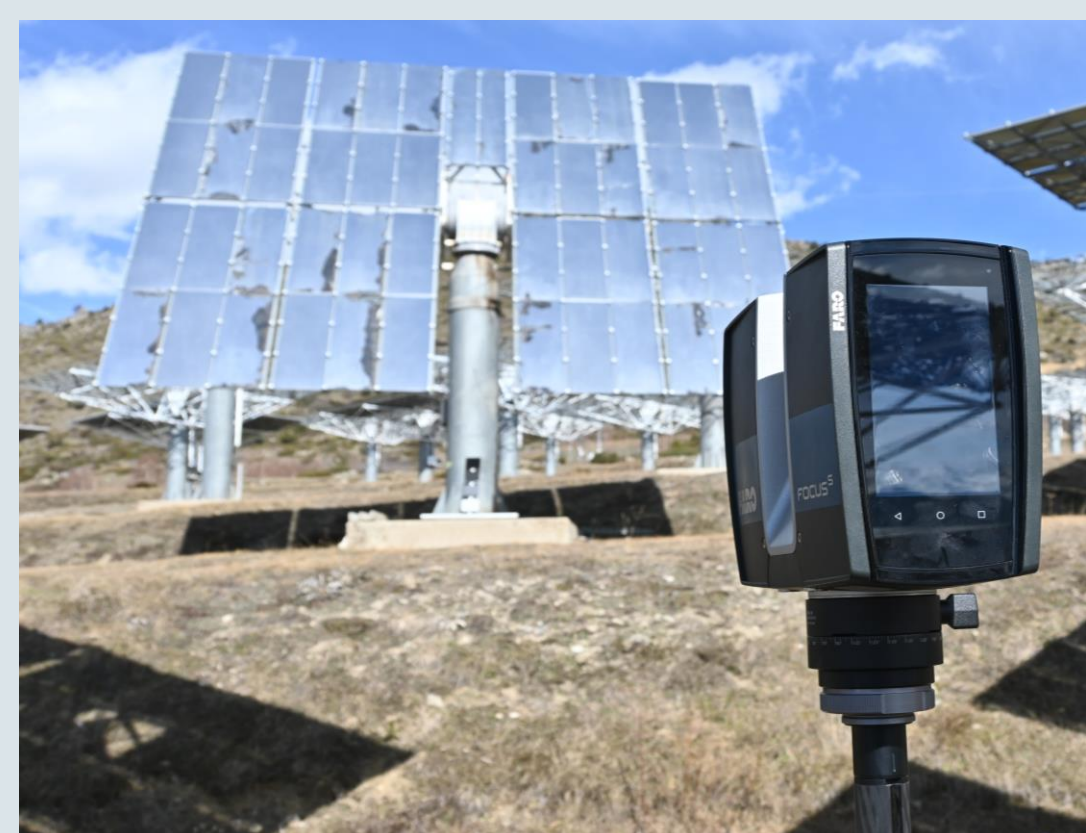
Figure 1. The Faro Focus S70 laser scanner captures a 3D point cloud of the front of a heliostat.
